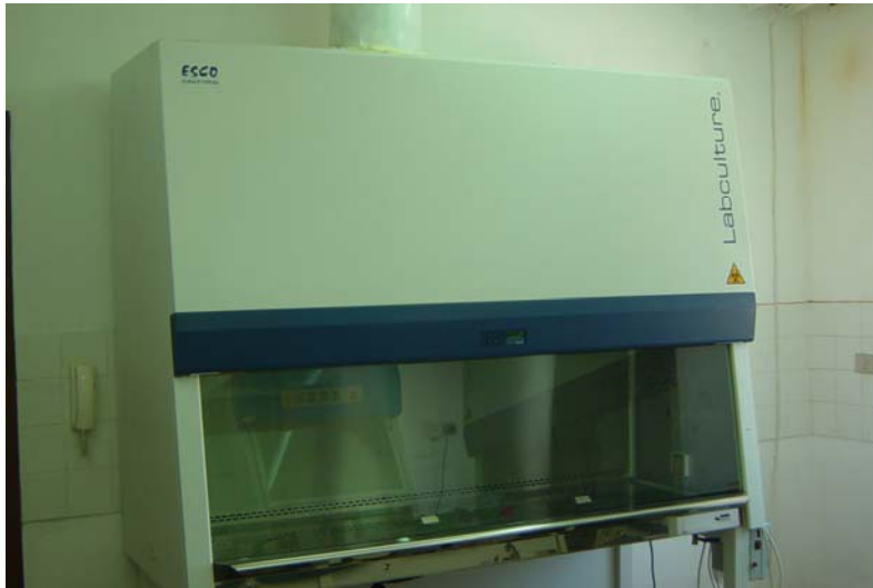
Safety Cabinet placed at NRL, Tirane
